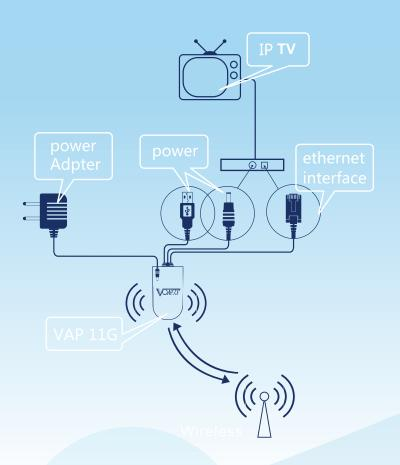
VAP11G is developed by HouTian Technology, is 802.11B/G WiFi bridge that is provided network cable specifically for the emerging IP monitoring solution. The main feature is as below:
